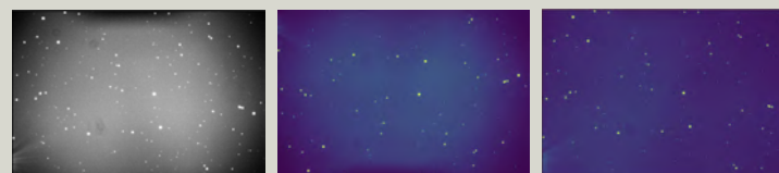
(a) Raw transit image of TOI-5451 taken on 4/7/2026. (b) Dark-subtracted image of TOI-5451 from 4/7/2026. (c) Fully calibrated image of TOI-5451 from 4/7/2026.
