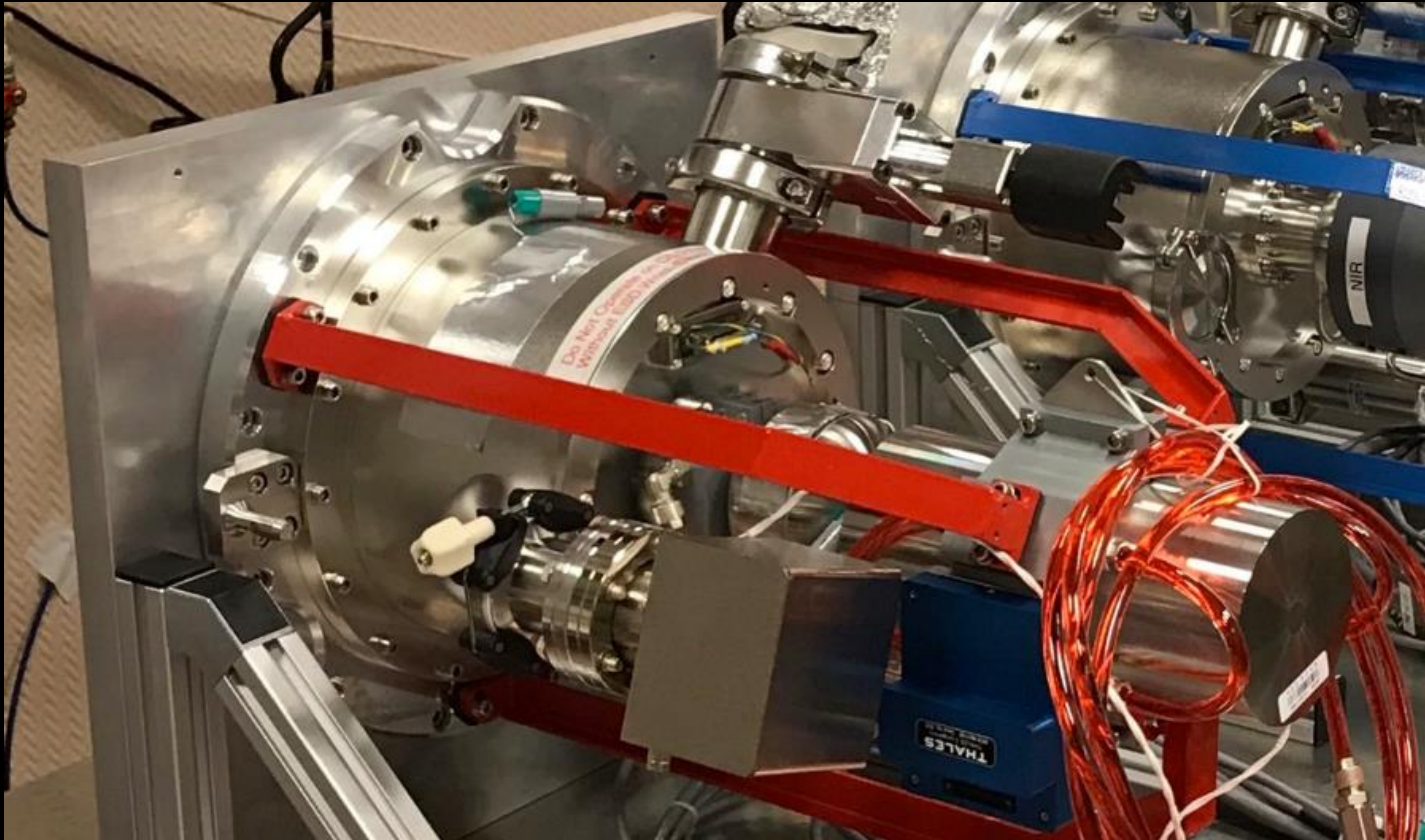
May 2017: Accelerometer on Spectrograph during vibration testing at Winlight.
