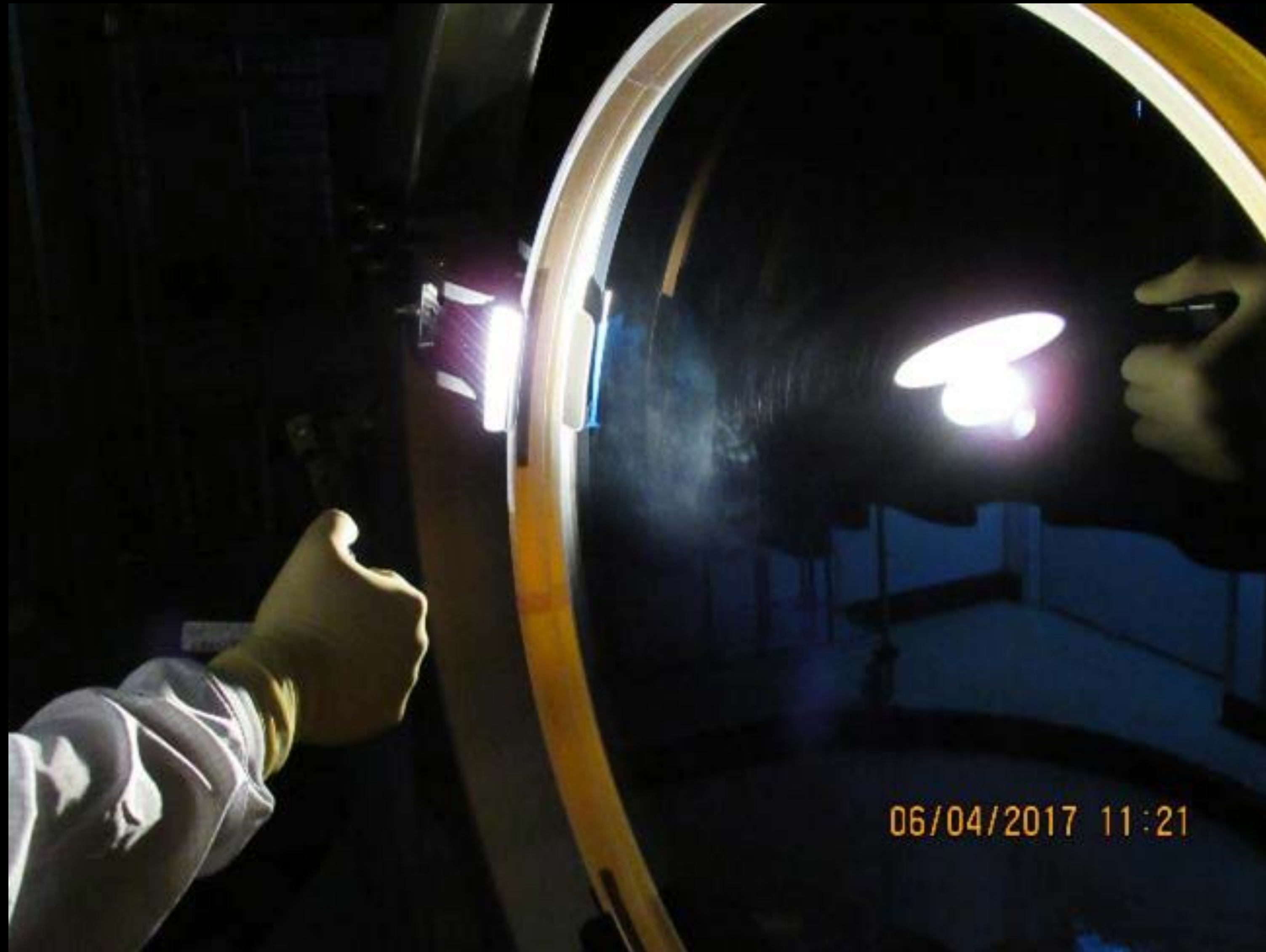
June 2017: Stain on side B of ADC2 is seen with a bright halogen light
