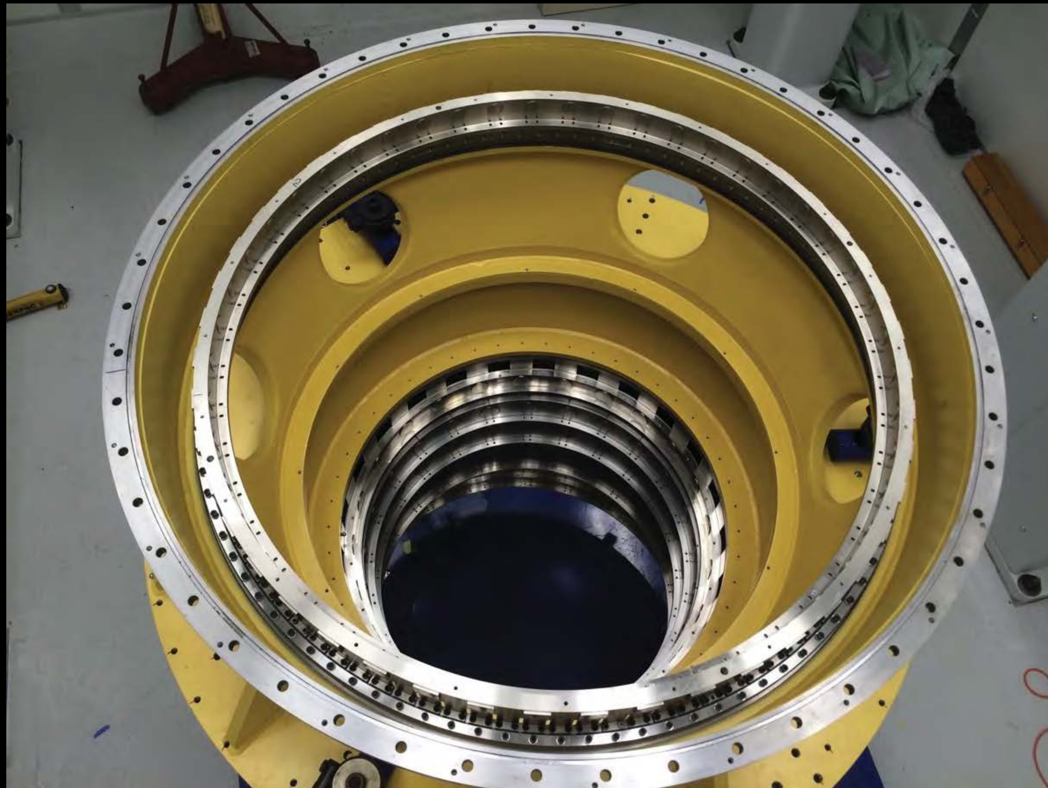
Nov 2016: Fully assembled corrector barrel at Fermilab aligns lenses to ~10 microns
