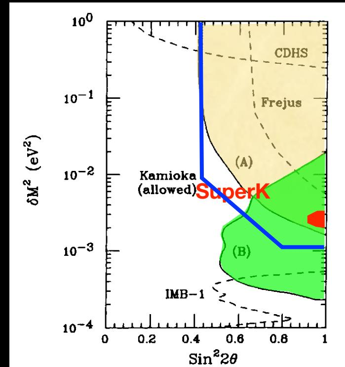
FIG. 2. 90% C.L. limits on  $\nu_\mu$  to  $\nu_e$  oscillations from rate (A) and stopping fraction (B). Dashed curves show limits from IMB-1 [14], Frejus [3], and CERN-Dortmund-Heidelberg-Saclay (CDHS) [15]. Dotted curve shows the allowed region from Kamiokande [16]. The Frejus limit is 95% C.L.; others are 90%.
