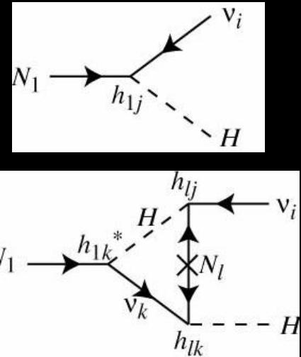
$$\frac{1}{\Gamma(N_1)} (\Gamma(N_1 \rightarrow \nu_i H) - \Gamma(N_1 \rightarrow \bar{\nu}_i H)) \propto \frac{1}{|h_{1i}|^2} \left( \left| h_{1i} + i\pi \frac{1}{16\pi^2} h_{1k}^* h_{lk} h_{li} \frac{M_1}{M_l} \right|^2 - \left| h_{1i}^* + i\pi \frac{1}{16\pi^2} h_{1k} h_{lk}^* h_{li}^* \frac{M_1^*}{M_l^*} \right|^2 \right)$$
