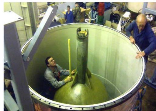
The intense EC source was lowered into the detector from above.
