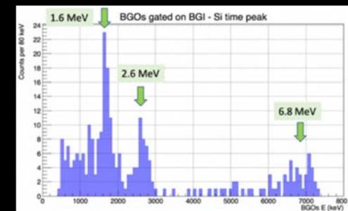
First recoil detection from  $^{16}\text{O}(\alpha,\gamma)^{20}\text{Ne}$  concludes construction
