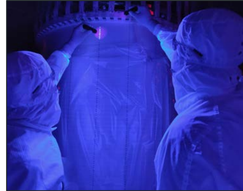
Inspecting for dust with UV light
