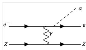
Figure 4: The Feynman graph for axion production through the electron-nucleus bremsstrahlung process.
