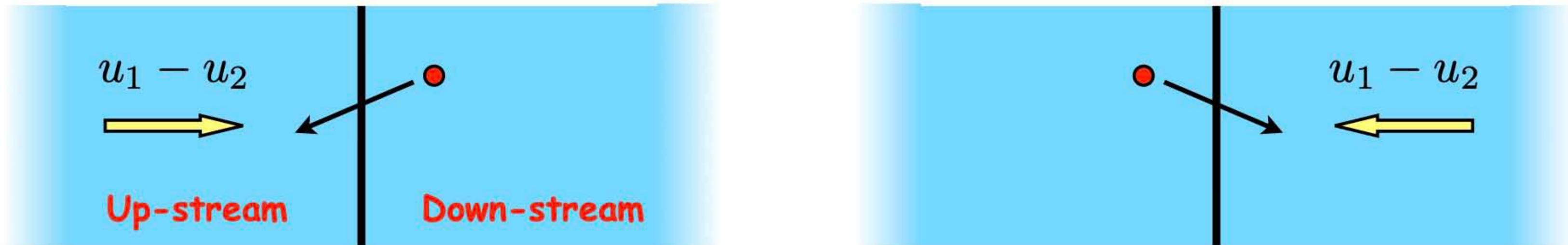
Every time the particle crosses the shock (up  $\rightarrow$  down or down  $\rightarrow$  up), it undergoes a head-on collision with a plasma moving at  $u_1 - u_2$ . Gain in energy at each crossing.
